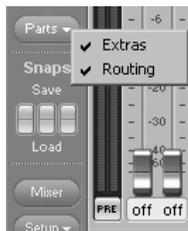
You may save certain visual configurations along with the current Output Control settings in a “snapshot”. For this, click on one of the three buttons beneath “snaps” on the row “save”. If you wish to recall a snapshot, click on the “load”-button situated beneath the previously saved snapshot.
