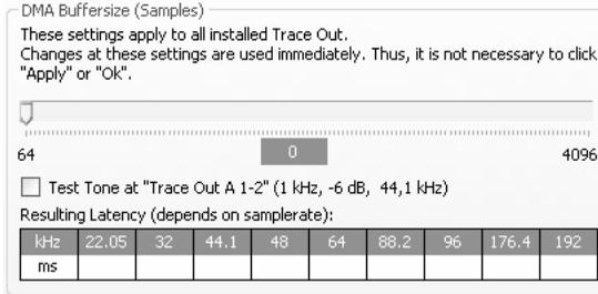
Via the upper slider you can adjust the minimal latency of the TRACE OUT. Here, the size of the buffer, shown in samples, is changed for the audio transport between PCI bridge and TRACE OUT. If you operate the soundcard with e.g. 44.1 kHz, 88 samples will result in a latency of around 2 ms. On 88,2 kHz, this number of samples would mean a latency of 1 ms. The cart “resulting latency” shows these connections for some important standard sample rates.
