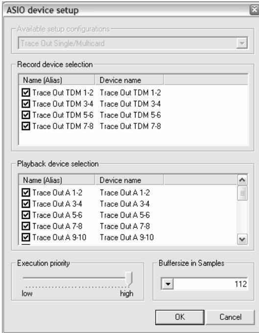
Due to small latency time, the ASIO interface has become a standard in professional music production. The ASIO device setup offers important settings for the TRACE OUT using the ASIO interface. It is opened from within an audio application, supporting the ASIO standard. Most times there is a button called “control panel” next to the field where the ASIO driver is selected – a click on it opens the ASIO device setup.
