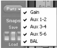
In order to adjust the look of the Mixer according to your needs, single rows of control elements may be hid or shown with the help of “Parts”. This applies to all gain-, aux- or bal knobs.
