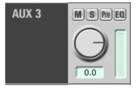
be switched on. A click on 'EQ' will make changes in sound as set up with the filters become audible on this mix sum.
