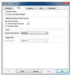
Working with digital audio signals, a digital clock is always required. The following settings define, which source is to be used for retrieving the clock for the SERAPH 8+  $^{39}$ .
