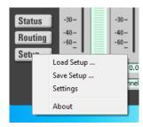
'Routing' calls up the routing window. From there again you can switch quickly to the mixer window via the 'mixer' button. 'Status' opens the clock status panel.
