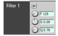
Each filter is full-parametric. That means, that it includes a graphical and numerical entry of the filter frequency 'freq' for
