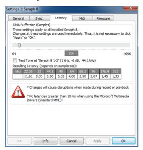
**DMA Buffer Size** Via the upper slider you can adjust the minimal latency of the SERAPH 8+. Here, the size of the buffer, shown in samples, is changed. Operating the soundcard with e.g. 44.1 kHz, 88 samples will result in a latency of around 2 ms. For 88,2 kHz, this number of samples would mean a latency of 1 ms. The chart 'resulting latency' shows these connections for some important standard samplerates.
