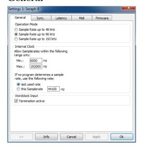
**Operation Mode** The SERAPH 8+ may be operated in 3 different modes, chosen here. In 192 kHz mode, the number of mixing sums must be reduced. There are then 2 aux-sums ('Aux 1' and 'Aux 2') besides the main mixing sum.
