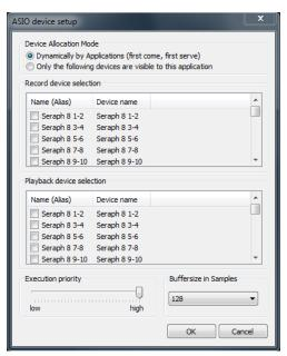
In the field of professional music production on the PC, the ASIO interface has established itself as a standard. The ASIO device setup offers important setup features for using the SERAPH 8+ with an ASIO interface. It is opened from within the audio application that supports the ASIO standard. Mostly there is a button called 'control panel' or 'setup' near the selection field for the ASIO driver. Clicking it will open the ASIO device setup.
